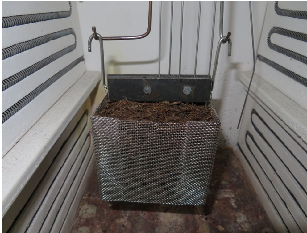
Figure 3. Basket Heating Test Setup.
